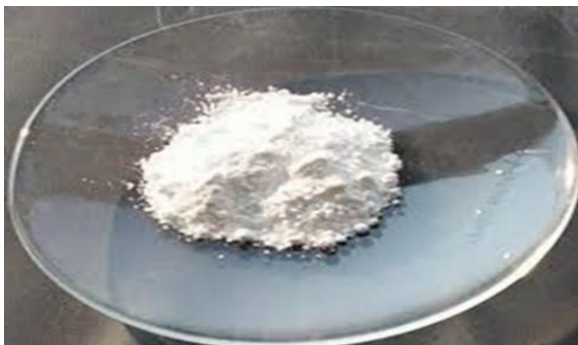
Fig.1: The image of calcined ZnO powder.
