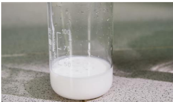
Fig. 2: The coating prepared by modifying ZnO particles with Stearic acid.
